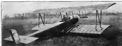
The plane for every occasion and occasion. Two seats—400 lbs. payload—40 hp. engine. Landing speed 20-25 mph. For more
